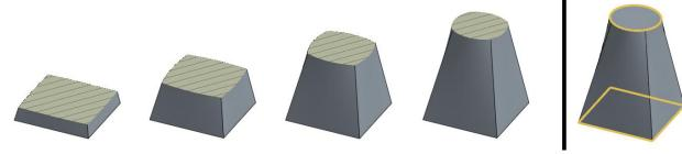
As we can see on the left, the cross-section (with the cross hatch lines) of the geometry slowly changes from a perfect square at the bottom to a perfect circle at the top.
